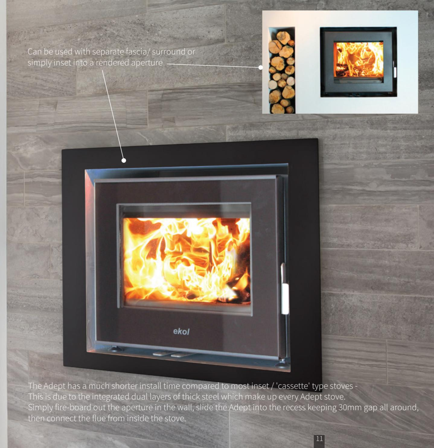
The Adept has a much shorter install time compared to most inset / 'cassette' type stoves - This is due to the integrated dual layers of thick steel which make up every Adept stove. Simply fire-board out the aperture in the wall, slide the Adept into the recess keeping 30mm gap all around, then connect the flue from inside the stove.
